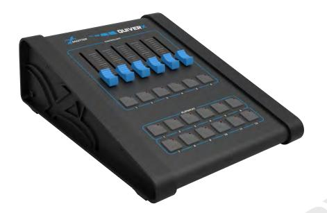
The QUIVERX expansion block was designed to increase the number of physical controller keys. The Expand is equipped with six faders, six button flash keys, 12 keys for direct access to playback registers, and one DMX universe through 3-pole XLR connectors. The QUIVERX expander can be easily connected to the mother console without any additional software, thanks to its dedicated cable that allows up to two expanders per console.
