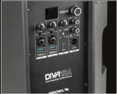
Two WIRELESS USB inputs for U24 microphone systems and BLUETOOTH STEREO TWS interface
