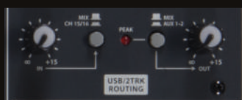
USB interface with routing options for PC recording and playback
