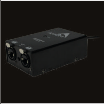
Dual-output USB to CAN converter
