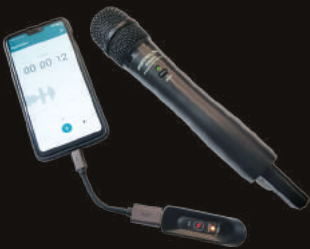
The U24 directly connects to PC, Mac computers or portable devices for digital stand alone applications.
